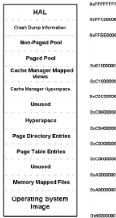
Fig 5. Normal system address space layout (*Intel*)
